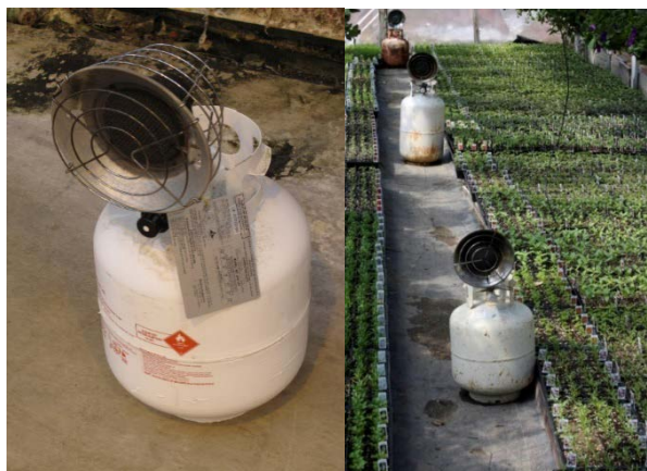
Figure 5. Unvented portable propane heaters should never be used in a greenhouse. (Photo: Roberto Lopez, MSU)
