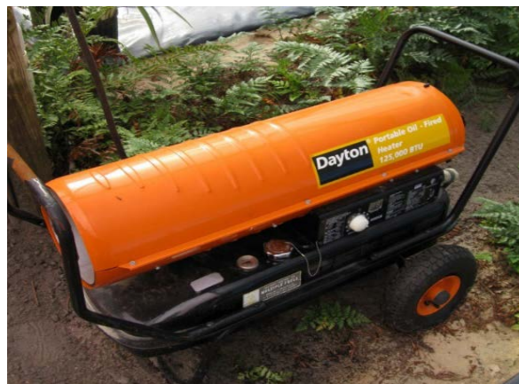
Figure 6. Unvented gas powered heaters should never be used in a greenhouse. (Photo: Roberto Lopez, MSU)
